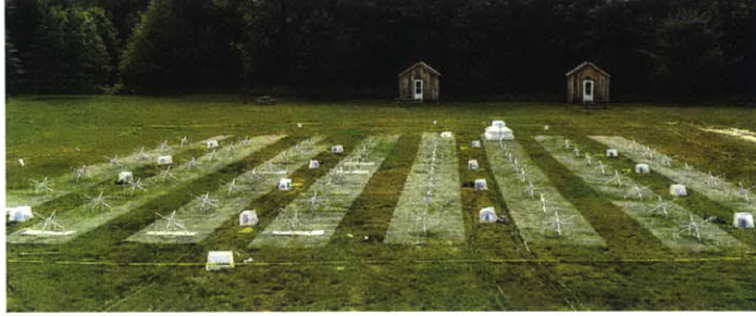
Figure 2-8: Part of the MITEoR array during the most recent deployment in the summer of 2013. 64 dual-polarization antennas were laid on a 21 m by 21 m regular grid with 3 m separation. The digital system was housed in the back of a shielded U-Haul truck (not shown).
