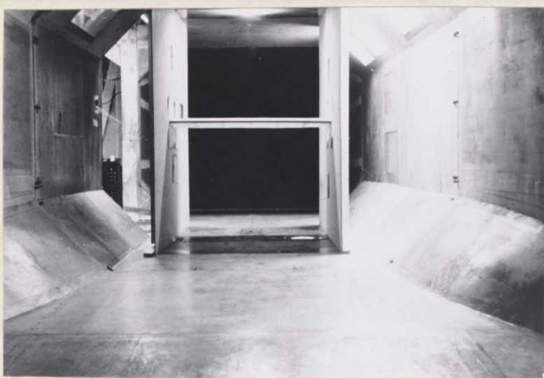
Fig. 3 Wing & Fairings Mounted in the Tunnel
