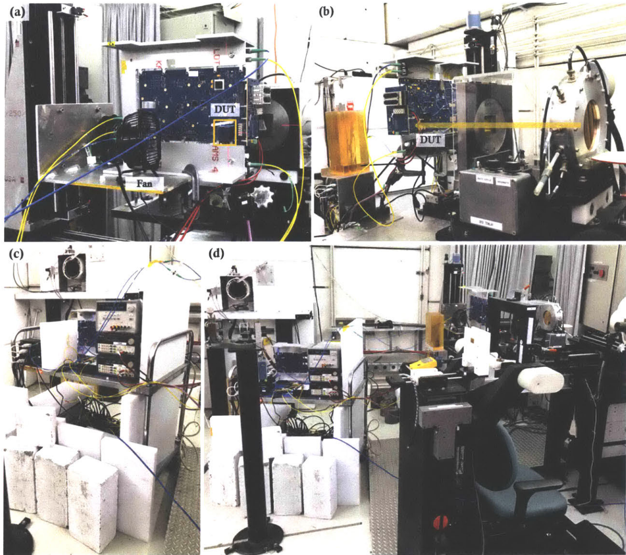
Figure 41. Optical coherent DSP ASIC proton radiation test setup. (a) OMA R-EDU mounted on radiation test stand with ASIC DUT aligned to center of proton beam collimator using laser alignment. (b) OMA R-EDU mounted for back-side proton radiation of ASIC through PCB. (c) Supporting test equipment, such as the GOMA R-EDU, test computers, power supplies, and optical-noise loading equipment, on a cart near the radiation test stand. (d) Full proton radiation test setup in the radiation chamber room.
