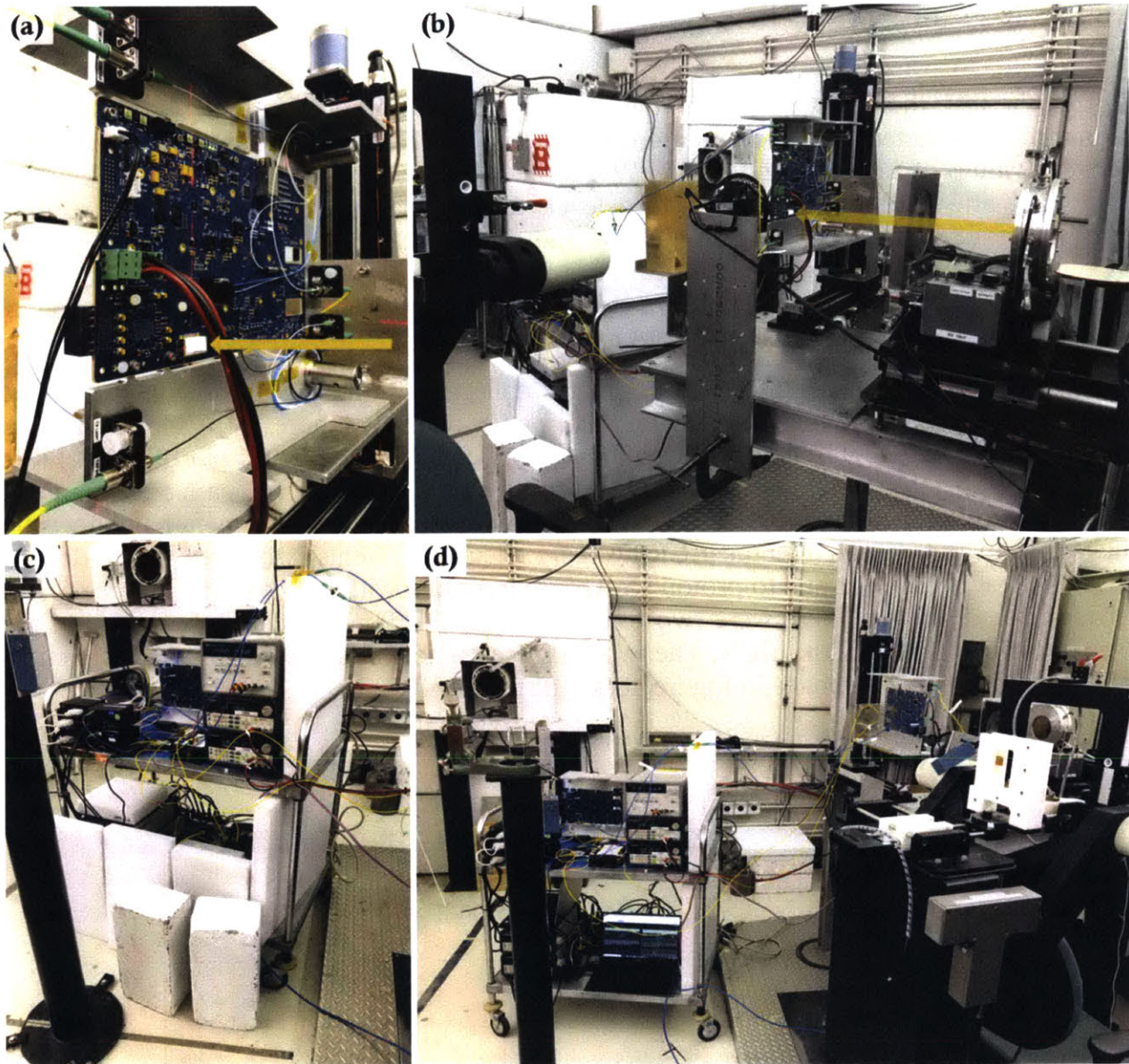
Figure 47. \mu ICR proton radiation test setup. (a) and (b) OMA R-EDU mounted on radiation test stand with top of \mu ICR DUT aligned to center of proton beam collimator using laser alignment. Yellow arrow indicates \mu ICR DUT on OMA R-EDU. (c) supporting test equipment, such as the GOMA R-EDU, test computers, power supplies, and optical-noise loading equipment, on a cart near the radiation test stand. (d) Full proton radiation test setup in the radiation chamber room.
