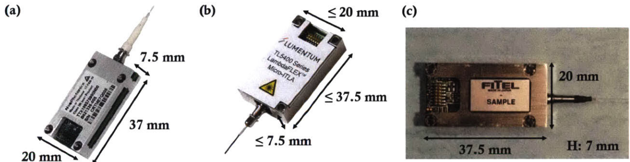
Figure 81. Commercial micro-integrable tunable laser assemblies from (a) Neophotonics, (b) Lumentum, and (c) Furukawa. [Lumentum, 2018; Neophotonics, 2018; Furukawa Electric, 2017]
