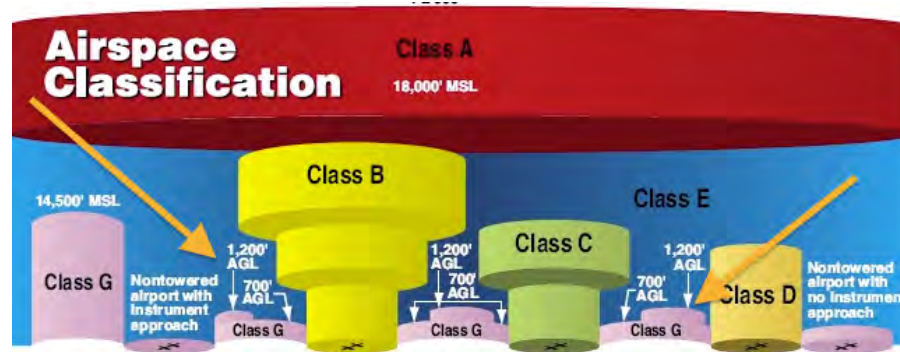
Figure 4: Airspace classification structure for U.S. NAS.
