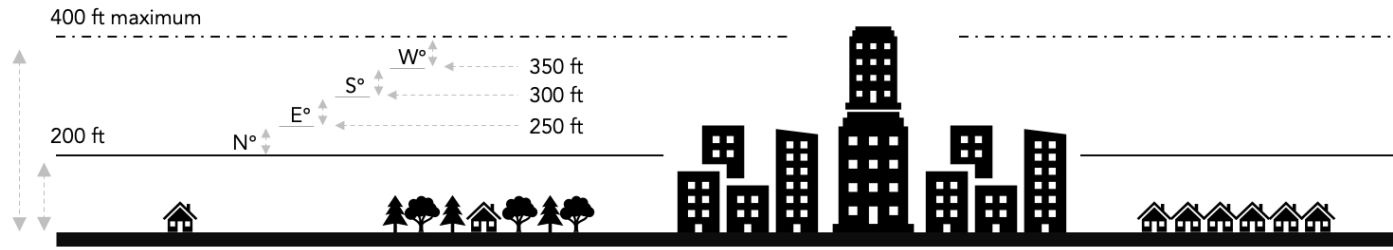
Figure 9: Graphic of proposed altitude stratification protocol for UAV-LMD.
