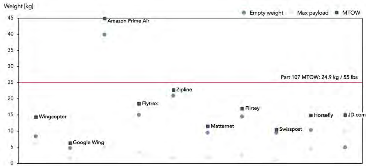
Figure 8: Survey of leading UAV-LMD industry leaders in UAV hardware empty weight, max payload weight and MTOW.
