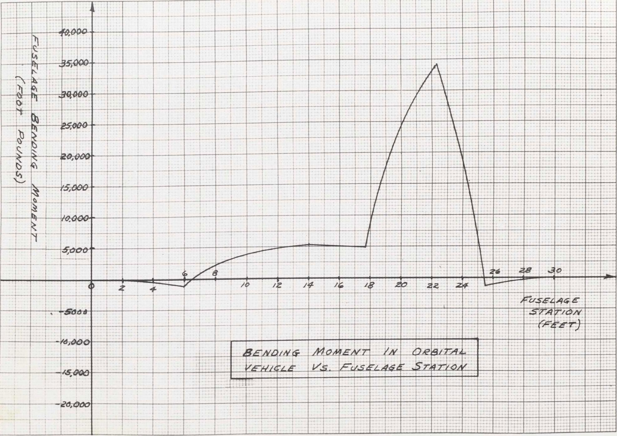
BENDING MOMENT IN ORBITAL VEHICLE VS. FUSELAGE STATION
