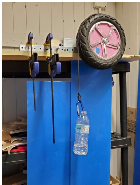
Figure 2-2: Measuring the motor's resistance to turning
