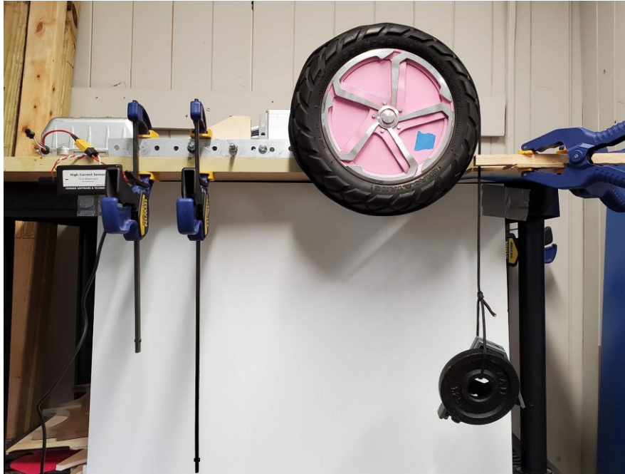
Figure 3-2: Experimental setup for measuring the efficiency of the Tailwind
