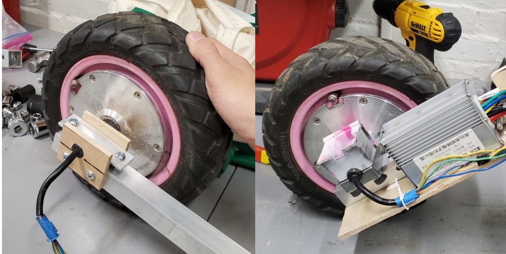
Figure 2-3: Old and new axle mounting solutions
