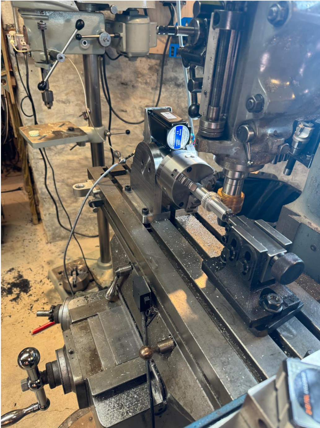
process of gear cutting
