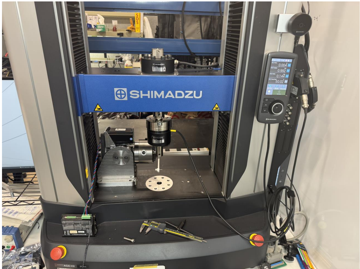
Figure 9. Stiffness testing on Shimadzu testing machine
