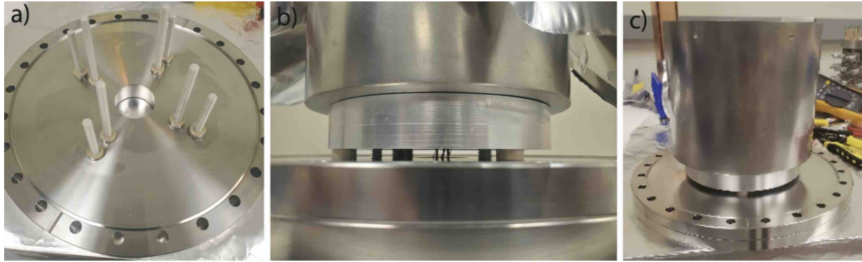
Figure 6.14: a) CF200 flange used to attach the VMI setup above the optical cavity. Four inner (4" long) and four outer (2" long) PEEK threaded rods are attached to the flange using previously made 1/4-20 threaded holes. 5 mm PEEK spacers are used to separate the flange (which is grounded) from the mu-metal shield (which is kept at a voltage of \sim -1 kV). b) An aluminum ring of 1" thickness is added between the flange and the mu-metal ring to compensate for a machining error on the length of the mu-metal shield. c) Top part of the mu-metal shield attached to the CF200 flange.
