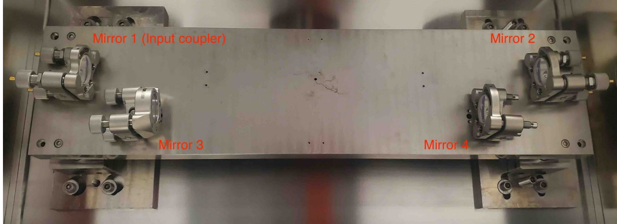
Figure 6.5: Bow-tie optical cavity used in our setup. The mirrors are labeled from 1 to 4, starting from the input coupler mirror. They are placed in THORLABS POLARIS mounts, with the two mounts holding the plane mirrors having piezos for fine adjustments of the cavity alignment once the setup is placed under vacuum. The cavity is placed on an invar plate (various holes in the plate are used to help with the initial alignment).
