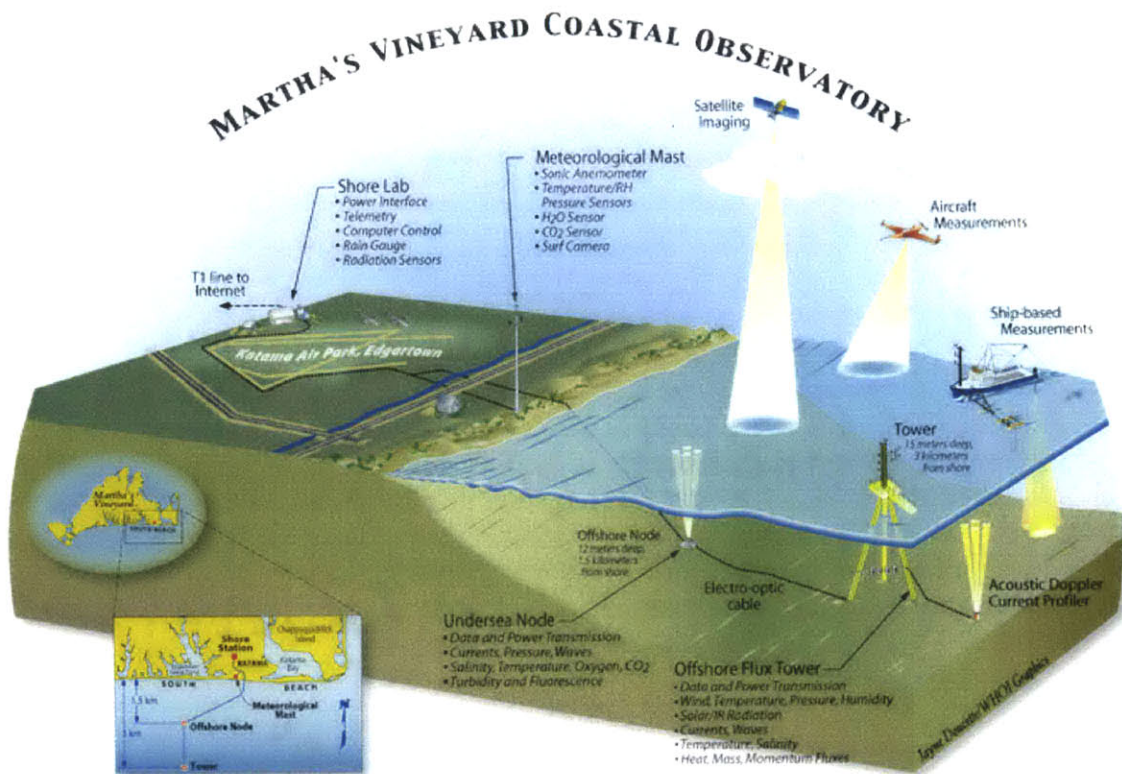
Fig 2.1 Schematic of the Martha's Vineyard Coastal Observatory, showing land-based, sea-based, and airborne components with available instruments and measurements. (MVCO website, http://mvcodata.whoi.edu/cgi-bin/mvco/mvco.cgi ).
