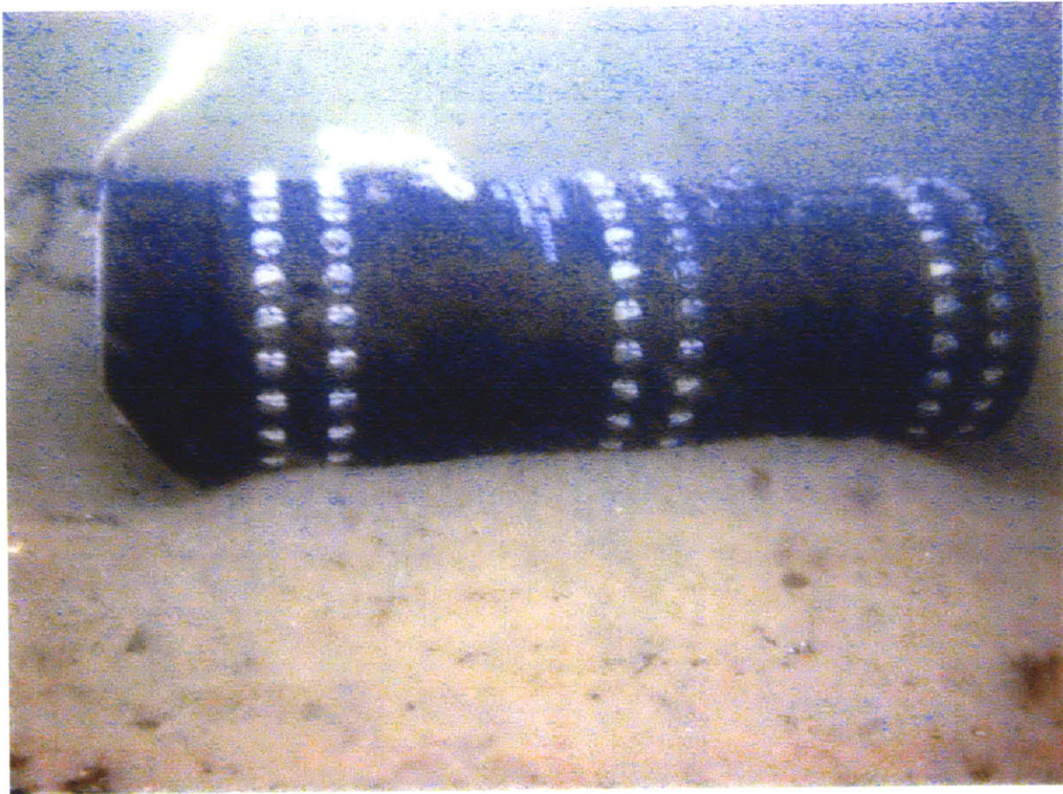
Figure 2.2 Optically Instrumented Mine (OIM) deployed at the Martha's Vineyard Coastal Observatory. The protruding optical sensor transmitter/receiver pairs are clearly visible beyond the hull of the mine. (Photograph by Richard I. Ray, NRL).
