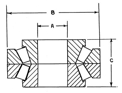
Figure 11: STEEP ANGLE TAPERED BEARINGS
