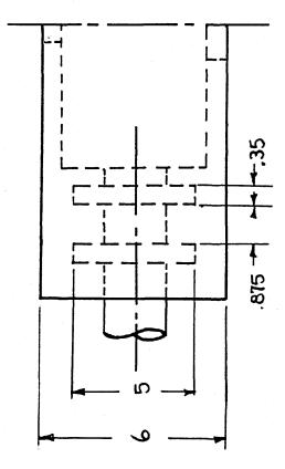
Figure 12: HUB, CROSS-SECTION
