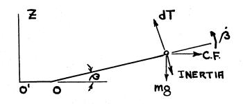
Figure 4: FORCES ON BLADE ELEMENT
