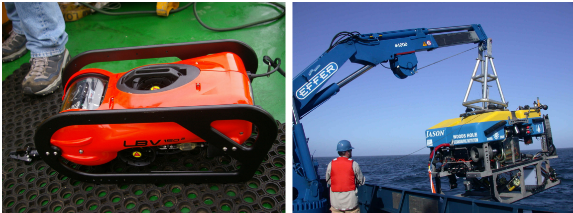
Figure 2-1: Seabotix 150 and JASON II ROVs (JASON II photo courtesy L. L. Whitcomb)
