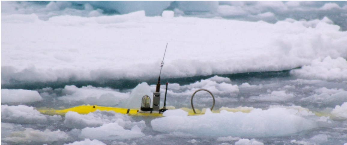
Figure 3-2: The Puma AUV sits in a small clearing in the pack-ice after completing an under-ice mission in the Arctic.
